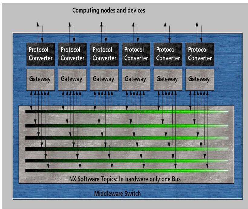
Figure 5: Logical view of the Middleware switch
